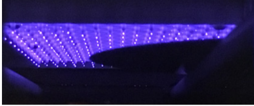
Figure 9. Wafer entering an EA zone for oxide removal
