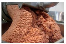
Almost by definition, food processing involves some form of heat, which needs to be removed before packaging or shipping. In meat processing, fats melt or soften under the influence of relatively little heat. With the high processing speeds required to be competitive today, more heat is generated during meat processing. This causes softening or melting of the necessary and desired fats and will result in a poor-quality end product.
