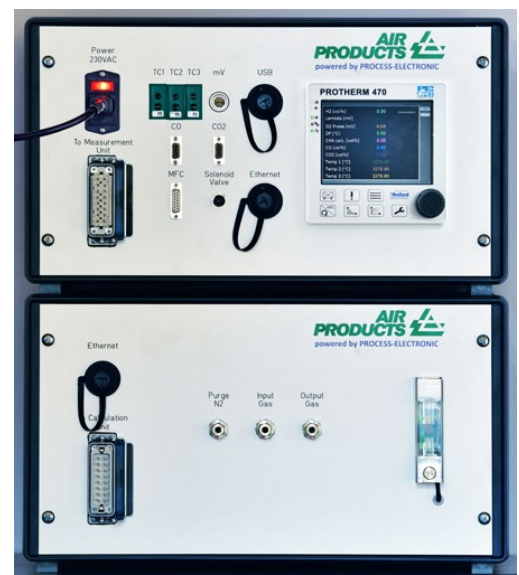
Air Products N 2 /H 2 atmosphere control panel
