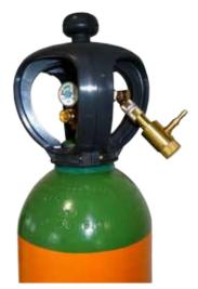
Specially designed for the Air Products 200 bar Integra cylinders. The dial-a-flow is adjustable in steps from 6-8-10-12-15-18-22-26-30 to max. 60 L/min.
