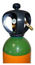
Specially designed for the Air Products 200 bar Integra cylinders. No need for extra regulators, as the outlet pressure (4 bar) and flow are preset. Simply change the optimizer and with one click you have the correct gas flow. The flow optimizers are available with a flow of 8, 10, 12, 15, 18, 20 and 25 L/min.
