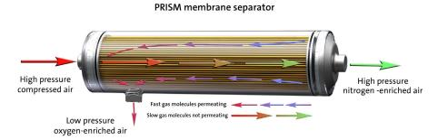
producing a dry nitrogen stream at the outlet. The secondary oxygen-rich stream is vented through a port in the shell wall.
