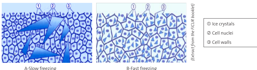
Figure 1: Illustration of crystal formation according to freezing kinetics
